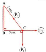
$\frac{F_1}{AB} = \frac{F_2}{BC} = \frac{F_3}{CA}$  $\therefore F_1 \colon F_1 \colon F_3 = 4 : 3 : 5$
